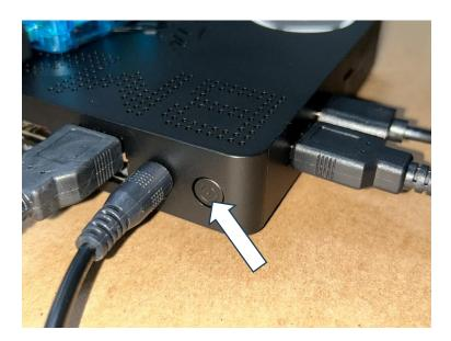
d. If step c didn't work, unplug the power to the main ECU. Use a paper clip to push and hold the hard reset button for 15 seconds. Then plug the power back in.
