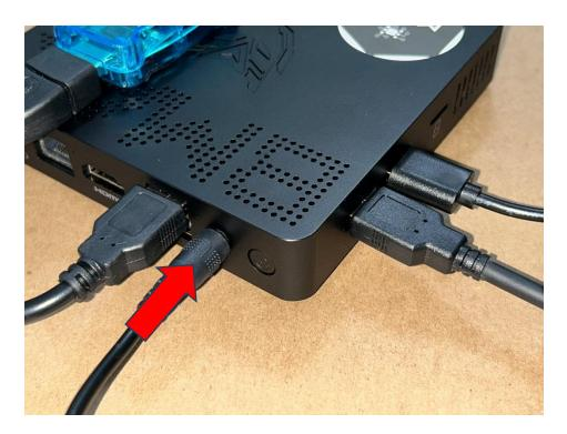
7. Once the power is connected, the system will auto turn on and boot up. This will take up to 2 minutes and you will hear the door lock release to let you know when it's ready to use. You should see a RED light on the relay, BLUE light on the main ECU, GREEN light on the card swipe and the QR should be flashing WHITE.
